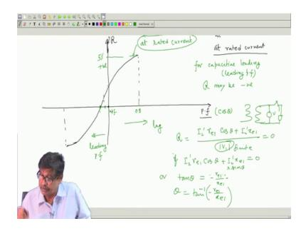
So, you sketch this curve in this way at least one curve I will sketch. So, this is the value of regulation, I will sketch percentage regulation. The regulation curve and this is suppose you sketch power factor and that rated current at sorry at rated current. Rated current means if secondary current is rated primary too will have rated current; you do not have to bother. So, load current is rated means primary side current is also rated.
