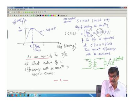
And we are discussing about how to estimate the efficiency of the transformer and if you see the previous lecture, this is the end result I have got that efficiency versus degree of loading. And we found out that efficiency will be occurring at maximum value at certain value of x; x as you know is a number between 0 to 1 equal to I mean full load condition.
