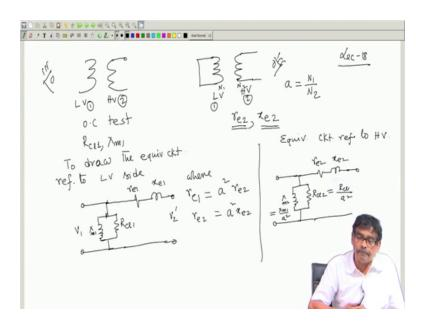
Now, after doing this test you see that I just draw here LV side, from LV side I carried out the OC test. And, whatever values you have got in the open circuit test this is the HV side; HV side was open. You got R Cl 1 the parallel branch and X m 1 this two values I got. And, while doing short circuit test which I told you for reasons not yet told that you suppose carry out the short circuit test from the HV side and during short circuit test you
