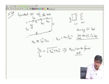
In this case the wattmeter reading, then approximately it records the copper loss, core loss can be neglected. During short circuit test some ways I right during SC test core loss it takes place no doubt is much much smaller then copper loss. Iron loss sometimes core loss is also called iron loss whatever it is much smaller. So, that can be neglected and we say the wattmeter reads the copper loss only.
