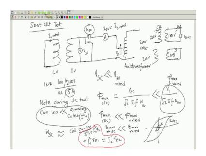
And, then if you carry out the short circuit test better carry it out from the HV side the reason we will discuss. But, if it is carried out from the HV side then what parameters you will get is r e 2 and x e 2 and the calculations are pretty simple.
