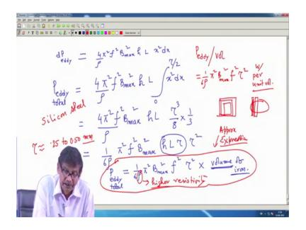
So, we got from the previous slide this is the thing therefore, this is the thing. Now the question is how to get P eddy total? So, P eddy total in that plate it will be equal to these are constant 4 pi square f square B max square into h into L and this is x square d x and this is to be integrated.
