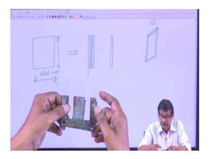
What I will do is this, this core material the this was the solid sectional area of the core this is solid iron. Instead of doing like this what I can do? I will take plates thinner plates and keep them side by side thin plates are you with me? That is the plates are like this you have you chop this thing with it cutting tools slices like your pages of book thickness of the book will be achieved.
