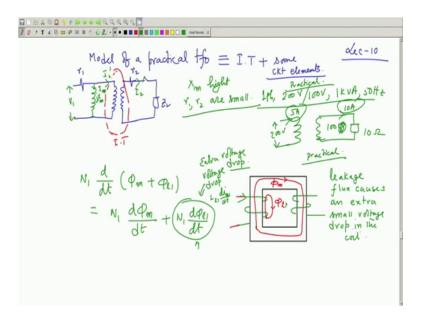
And I told you that till now what we have done is, we have added the winding resistance  $r \ 1$  of the primary and this is my ideal transformer and here is your actual load on the secondary side z 2, and here also I showed the secondary resistance  $r \ 2$ . And then the magnetizing current was also taken into account and it was not a winding, it is x m, it is my thought process which brought me here. This is my applied voltage.
