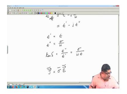
So, culprit here is the presence of this conductivity that is why the epsilon is effectively called a thing and so, we define that loss tangent is given by epsilon double prime by epsilon prime and that is sigma by omega epsilon.
