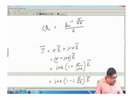
And the angle theta n the angle of the intrinsic impedance that is tan inverse sigma by omega epsilon by 2 and so. The current density, that since its still in Ohm's law abiding case. So, we can say this is the conduction part and this is the displacement part. So, it becomes sigma plus j omega epsilon in to E. So, we can take j omega epsilon out and that gives us 1 plus sigma by j omega epsilon into E and that we can write it as 1 minus j.
