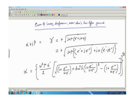
So, we will see that now that when e m wave falls through ground we can again redo the e m theory cases I am not going into that; but we need to determine the attenuation constant. So, the case of ground I can say the case of lossy dispersive non Ohms law type ground. So, we here we cannot assume anything; so but in all these cases we can go to our basics. And say that what is the propagation constant gamma?
