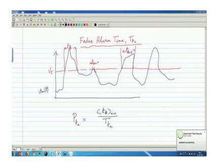
So, we were discussing the false alarm time T f a and you can refer to your graph I have drawn it again the same thing. So, we were we ended here that probability of false alarm is equal to the time that the noise voltage stays above the threshold average of that by T f a.
