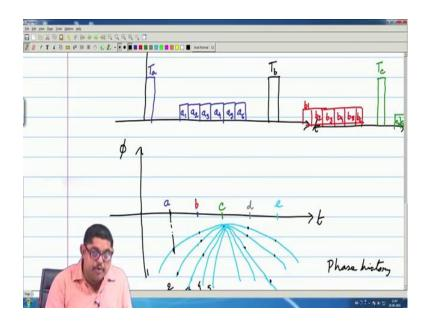
Let us say the time diagram. So, radar at let us say this point is sending a transmitted pulse T a. I am calling it T a that a subscript. So, if I now see these in response to this from different range bins, I can consider that one this bin the; that means, one this rectangular portion that is an object. So, for me this is the resolution that the whole thing in this range they will give a return. Let me call that return as A 1; similarly from the next range bin I have got the return A 2.
