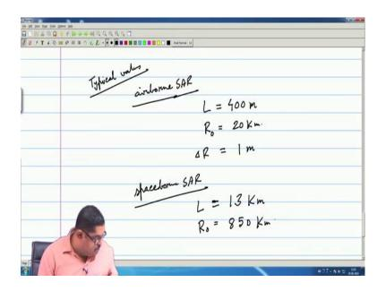
Now, there are generally two varieties of SAR one is airborne SAR. Airborne SAR means the radar is flown with a on an aircraft and aircraft moves. So, typically I can take some typical values of Indian made SARs the synthetic aperture length is 400 meter, the range R naught is 20 kilometer. So, in that case the delta R that will come to be 1 meter.
