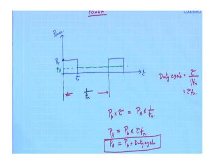
So, let us come to the next thing that what is the transmitted power of the radar? So, for that we have already seen this time domain picture of the transmitted pulse. So, we are sending pulses one by one. So, here let us say now the; this diagram this is time, this to calculate power; this is our power. So, let us say that the; this is the previously I was calling this as amplitude domain. So, power will also be similar type of curve and let us call that this pulse pick power that is P p.
