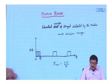
You see so, first let us say the basic definition is the shortest distance of the target shortest distance or shortest range of the target you can say in better shortest range of the target detected by the radar. So, this is called your minimum range. Now in a pulse radar, we are sending; we have seen that the at a pulse repetition frequency, we are sending the thing now let us say that the on time of this.
