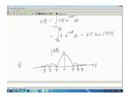
So, I will have to now find the H f. So, H f is minus Fourier transform h t e to the power minus j omega t dt. So, this is it exists from minus tau by 2 to plus tau by 2 ht's value is A. So, it is A e to the power minus j omega t dt. So, this we know simple to integrate A tau sinc pi f tau so, as easy as these.
