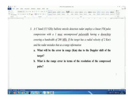
Let us see the last problem. This is a problem A C band ballistic missile detection radar employs a linear FM pulse compression with a 1 millisecond uncompressed pulse with having a down chirp covering a bandwidth of 200 Megahertz. If the target has a radial velocity of 2 Kilometre per second and the radar mistakes that as a range information.
