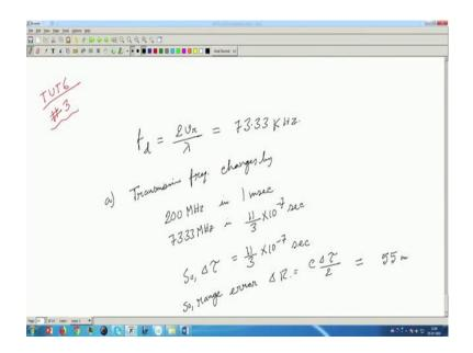
So, first find out the Doppler. So, radial velocity said the frequency said. So, you can calculate this will be 73.33 Kilohertz. Now, first is you see the due to LFM the transmission frequency changes by 200 Megahertz in 1 millisecond.
