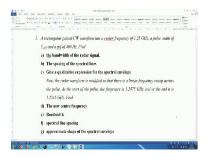
First problem is this detect. A rectangular pulsed CW waveform has a center frequency of 1.25 gigahertz a pulse width of 5 micro second and the prf of 400 hertz. Find the bandwidth of the radar signal, the spacing of the spectral lines, give a qualitative expression for the spectral envelop. Now, the radar waveform is modified.
