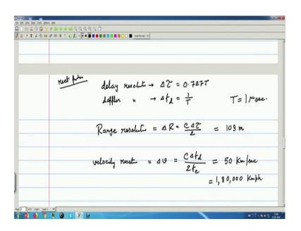
So, I can write now that delay resolution this is for rectangular pulse we are still discussing that rectangular pulse. So, delay resolution is; that means, delta tau that is 0.727 T and the Doppler resolution that is delta f d that will be 1 by T.
