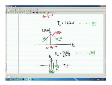
And here we can find what is the peak value again the peak is same you see here also the peak is a square root over 2 pi sigma square and this 3 dB points. So, let me call that 3 dB point W 3 in frequency. So, that W 3 if you calculate it will come as 1.662 by 2 pi into 2 sigma. So, this is our equation number 48.
