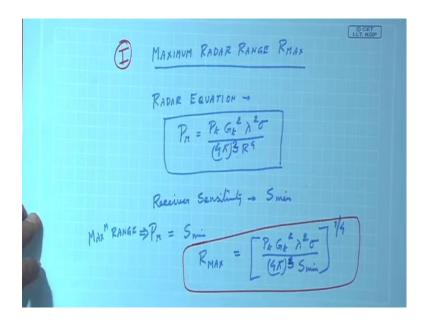
Today we will see, the first parameter that what is the radar range maximum range of a radar; that means, given a radar system with its transmitter, with its antennas etcetera and given a target with its radar cross section. And obviously, when I have given a radar system it has a transmitting frequency.
