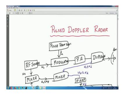
So, this was the block diagram of pulse radar, the same thing was there in the pulse radar. So, there you see that the received signal after the antenna receives it. So, we get it here the here you see the antenna. So, through duplexer it is coming and it is put to mixer. So, RF mixer mixes that and makes the IF signal. Now this IF amplifier we used to say today we will see that what is the IF amplifier implementation actually radar people call these match filter.
