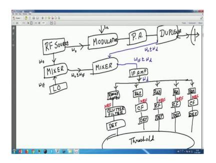
And to start with this discussion I refer you to the previous block diagram of pulse radar pulse radar or pulse Doppler radar.
