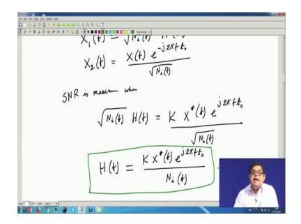
So, we can say that SNR is maximum when root over N i f H f is equal to sum constant K into X star f e to the power j 2 pi f t naught divided by root over N i f.
