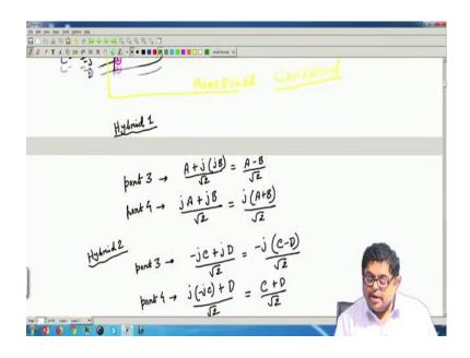
I can say at port 3, I can write hybrid 1. So, I can write the port 3 will be that A plus j into j B by root 2. So, this is nothing, but A minus B by root 2.
