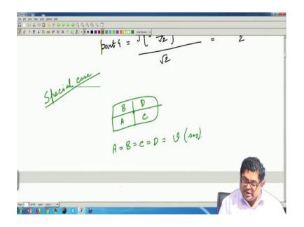
And let us check that whether my circuit is ok, we can check by giving a special case. What is that special case that let us say; that the target is on the boresight or target is on the monopulse axis. So, if the target is on the monopulse axis; that means, if these are the four feed horns; so, target is here at the center. So, what will be the value of A B C D; we had A B C D.
