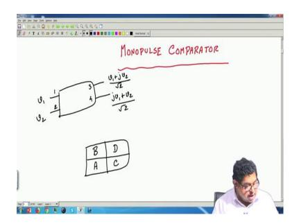
Then I am just for recapitulating this will be required. So, what we have seen that if we have a either hybrid or a coupler that the requirement it should have the port 1 and 2 as a input port and port 3 and 4 as a output port and if we give signal v 1 here if v 2 here and then this 3 that is v 1 plus j v 2 by root 2 I am using a top-wall coupler.
