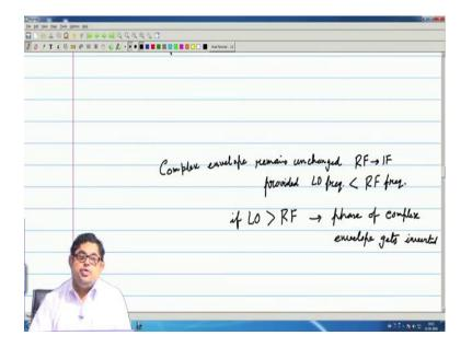
The complex envelop the complex envelop remains this can be proved remains unchanged when we make RF to IF conversion. But, there is a catch actually generally in communication this catch always is not mentioned that, this is true remains unchanged provided a LO frequency local oscillator frequency is below RF frequency. And if it is not if LO is because I can make LO also greater than RF also the then the phase of complex envelope gets inverted.
