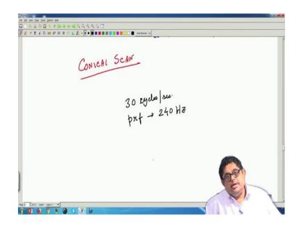
Conical because any antenna can be if you want to have both traverse and elevation information, then it should be rotated in the conical scan. So, beam motion is continuous in conical scan, but target gets illuminated only when each transmitted pulse reaches it. So, typically the antennas scanning rate is 30 cycles per second etcetera and suppose my prf typical prf we have seen of a pulse radar 240 Hertz so; that means, you can say that for one complete scan I will have 8 beam positions.
