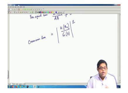
So, this loss is called crossover loss due to shifting to; that means, I am shifted to so, here we need to quantify this. So, suppose the squint beam it is at a position minus theta naught. So, what is minus the naught the maximum position. So, since it is shifted to this side I am calling it minus theta naught if it had been shifted to this side that would have been plus theta naught. So, crossover loss is what? You see how much power loss is obviously, power.
