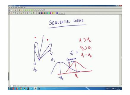
So, we will discuss sequential lobing. So, you have two fixed beams now you see that one antenna, antenna can be designed properly so, that it can have multiple number of beams. So, we are not always; that means, an antenna please remember, an antenna can have multiple beams. So, what we will say that in sequential lobing whether a single antenna or multiple antennas, they produce two squint beams.
