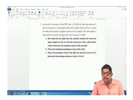
So, this is an interesting problem an aircraft is carrying an L band MTI radar for detecting rainstorm. It detects rainstorm in its path approaching with a relative velocity of 12 meter per second. So, you know that CW radars there used for detecting rainstorm. It is having an MTI facility.
