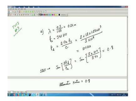
Tutorial 3 problem number 3. So, first it is a L band radar. L band you know 1 to 2 giga Hertz. So, this is given as 1.25 giga Hertz. So, that is lambda will be then 0.3 by 1.25 that will be 0 point; that means, 24 centimeter is the lambda. Okay also it is said that relative velocity the prf of the radar transmitter is 340 Hertz. So, prf is 340 Hertz and radial velocity given we can calculate fd. So, fd will be 2 vr f naught by C.
