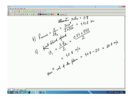
So, let us we can see the question, then part b is what is the maximum unambiguous range of this radar. So, that will be our next step. The maximum unambiguous ranges are unambiguous that is c by 2 fr so, that we can put the value 2 into 340. So, that will give us 441.2 kilometer; that means, our unambiguous range is 441 kilometer and what was the part c, what is the maximum velocity with which the aircraft can move if it is known that the maximum rainstorm velocity is 20 meter per second?
