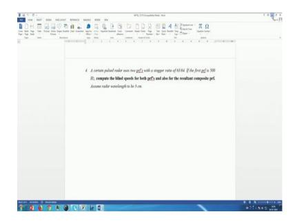
Then this problem, a certain pulse radar uses two prf s with a stagger ratio. So, prf staggering we have discussed it is a question on that with a stagger ratio of 63 64. If the first prf is 500 Hertz, compute the blind speeds for both prf's and also for the resultant composite prf. Assume radar wave length to be 3 centimeter. So, let us see the solution. So, stagger prf so, we will have to find blind speed for each prf and also for the composite prf when you have staggering.
