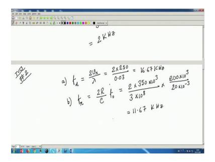
Problem 2, tutorial 3; so, the first part says that the mean Doppler shift, now what is Doppler shift? fd is equal to 2 vr by lambda. So, vr which has been said that radial velocity 250. So, 2 into 250 by lambda is 3 centimeter that is 0.03. So, that gives us 16.67 kilo Hertz is the fd and fb up so, fd is known. Now fr, what will be fr? fr the same formula we will use 2 R by c. So, these values as said, the frequency target is at a range of 350 kilometer.
