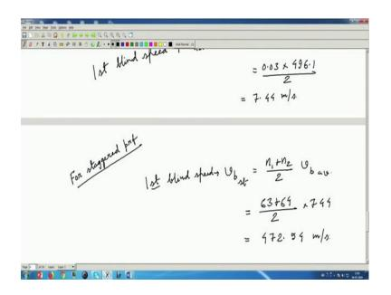
Now whereas, so, this is a average constant prf, but for staggered prf for staggered prf, first blind speed formula we know first blind speed if we call that fb staggered; that is n 1 plus n 2 by 2 vb average. So, that will be 63 plus 64 by 2 into 7.44. So, that will be 472.54 meter per second. So, you see that staggering is qualitatively changing the game.
