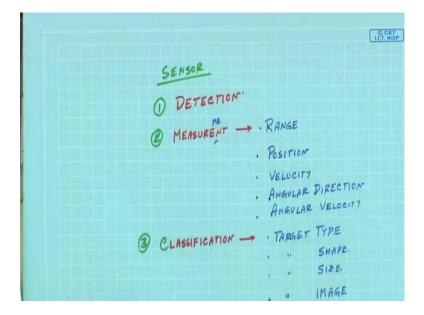
Now what are the primary functions of radar? First thing is as the name suggests that if the primary function of this is detection. There is no doubt about it that I will have to detect whether there is an object or not.
