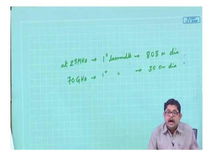
So, the fall out of these is that suppose at 25 mega Hertz; at 25 mega Hertz, to get a 1 degree beam width because why I need smaller beam width? Because beam width means in that portion my maximum power is concentrated. So, suppose if I want to detect something, if I can localise the power then I am making efficient use of the power.
