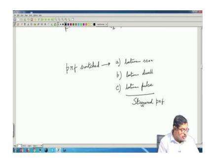
Now so, we can say that instead of two radars, 1 radar can multiplex the 2 PRFs now there are various ways by which this can be done. So, we can say PRF switched; PRF can be switched one scheme is between scan; that mean, in one scan you know antenna scans so, in one scans the PRF is something and the next scan it is a different PRF, then some radars they do it between dwells. Dwells means when you are at a particular beamwidth; that means, when you are scanning 1 beamwidth scan is called dwell.
