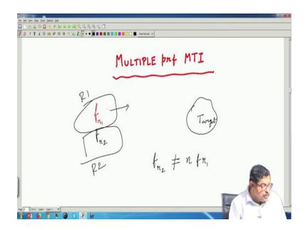
So, now, to understand the concept, first think that there are two pulse radars with different PRFs suppose, PRF fr 1 and another PRF is fr 2 and they are trying to detect a target. So, obviously, since so, this is one radar; radar 1 and this is another radar; radar 2 they are trying to detect the same target. So; obviously, the first blind speed of this radar is different from the first blind speed of this radar, because their PRFs are different.
