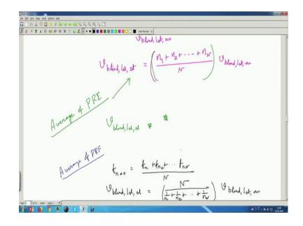
So, if we do that, so we can make the relation that v b or blind v blind first stagger is nothing, but n 1 plus n 2 plus n N by N into v blind first average.
