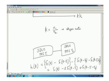
So, if we have that so that means, I have a I can say one SDLC with PRI T 1 and then another SDLC with PRI is T 2. So, this will make a three-pulse canceller. So, we can easily write what is the impulse response; that it is delta t minus delta t minus T 1, then delta t minus T 2 minus delta t minus T 1 minus T 2. So, we know it is delta t minus 2 delta t minus T 1 plus delta t minus T 1 minus T 2.
