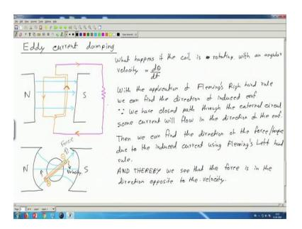
So, then normally there is no current. So, normally there is no current, so, the coil will not move normally, but if the coil starts to rotate due to any reason, if the coils say if the coil is moving, then what happens. So, the question that we are going to ask is what happens if the coil is moving or rotating. Say the coil is rotating in this direction; I am just choosing a direction arbitrarily.
