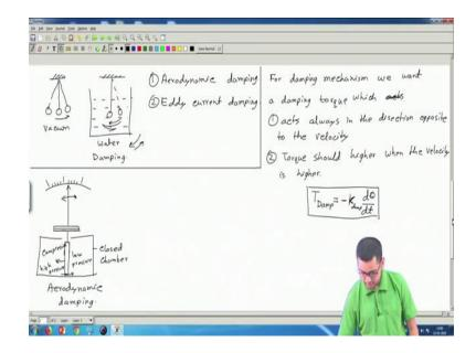
So, this is in vacuum and I move it in either direction, then this will start to oscillate. And, this will keep oscillating, maybe forever because it is in vacuum there is nothing to stop it there is no energy dissipating reason to stop it, there is no friction nothing.
