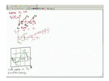
So, let us draw V V. V V will look like this, time versus V V. This I will take it like this, I will take it like a sine wave which is like this. It completes one cycle in exactly same time as it is taken by this horizontal voltage to complete one cycle from negative to positive, this is this is one cycle, this is also one cycle.
