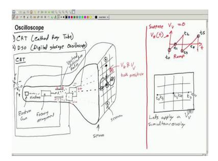
So, let us start with CRT which is which means cathode ray tube oscilloscope, ok, so this is one type. Another is DSO digital storage oscilloscope. So, let us talk about first how a CRT works? All of you might have seen this in your lab, but let us know what is there inside and how it actually works. This is made up of mainly hollow tube like this, ok. So, this is a glass tube and this is evacuated.
