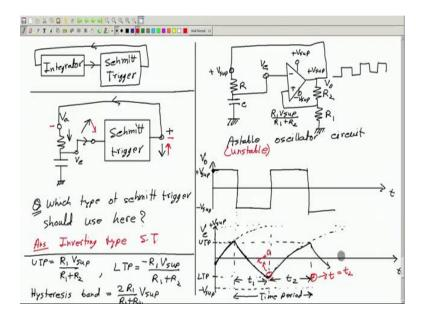
So, recall this, so in one of our circuits we had a Schmitt trigger and integrator and we connected them in a loop. The output of the Schmitt trigger goes to the integrator; therefore, the output of the integrator changes continuously, it increases or decreases and at some point, it triggers this Schmitt trigger to change its output. And this way this entire system oscillates between two stages, two states.
