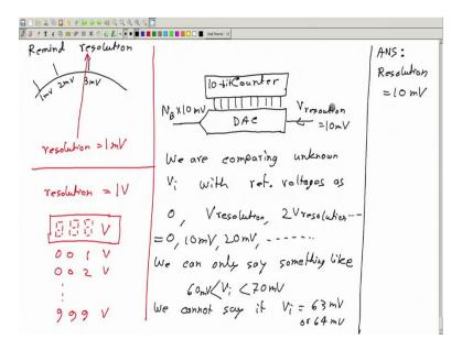
So, before that let me just remind you what resolution is? What do we mean by resolution? If I have say a voltmeter, which has markings like this 1 millivolt, 2 millivolt, 3 millivolt, etcetera and it has a pointer definitely. So, the point, this is the pointer. So, the pointer can be here, here also in between; but it has only these markings.
