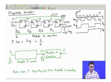
So, let us talk about it so, frequency divider. What is it? This is nothing, but a counter we have seen it ok. So, do you recall that we have drawn a ripple counter like this, which is made up of a number of T flip flops toggle flip flops and these are the T inputs of all these flip flops, these are their outputs and we have clocks these are negative edge triggered T flip flops the way.
