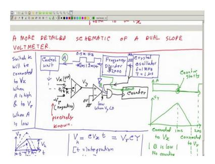
And, so, there were a few small blocks ok, like a frequency divider and integrator most importantly and comparator. So, these we have drawn as block diagrams. So, we should also know how they are made or how they work? Now, comparator we already have started in much detail.
