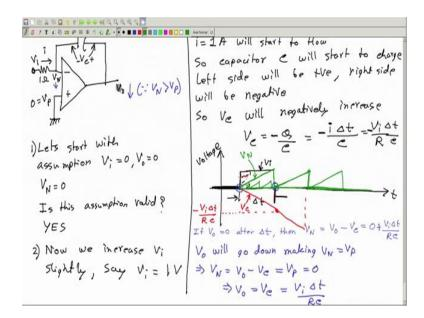
So, let me draw the circuit once again ok. See, we will start the analysis with the assumption that V i. So, let us start with the assumption that V i = 0, V o = 0, and this is V N, V P; V N = 0, V P = 0 this is not an assumption this is connected to graph this is V i.
