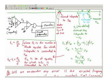
So, actually we do not have the value of t 1 or t 2. What we have is this; I mean, we actually have t 1 = C1/f where, C 1 is the counter value at this point, ok. Say, say if the counter starts here ok, then it will be the value of the counter here or I may also start the counter here I may not so, I withdraw my last statement that may be confusing.
