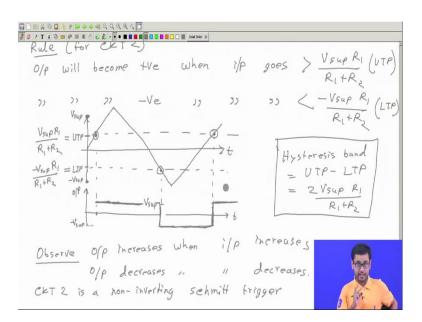
The rule for circuit 2; output will become positive when input goes above this V supply R 1 goes above V supply R 1/(R1 + R2). Similarly, output will become negative when input goes let us see it is written here minus V supply R 1/R 2; below so; that means, this I can call the upper trigger point; this I will call the lower trigger point ok.
