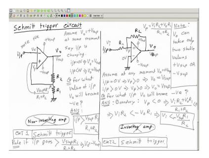
So, the topic is Schmitt Trigger circuit; you may already call that in an additional video we actually have seen this while studying op-amps and I just have mentioned that Schmitt trigger is nothing, but wrongly connected amplifiers inverting or non-inverting amplifiers ok. So, we found it like that let us first draw inverting and non-inverting amplifier.
