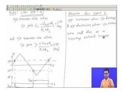
Output becomes positive if or when input goes below and output becomes negative when input goes above ok. So, let me draw some diagram time versus say input say the input is changing like this; maybe a triangular wave, you can also use sine wave and say this height represents the value of this V supply ok.
