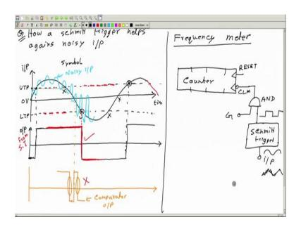
So, what are we discussing now? So, we are discussing how a Schmitt trigger helps against noisy input ok. So, if the input signal is noisy like this. So, this is an ideal sine wave, but see the input signal is actually like this, it is noisy and let me make it a bit more noisy ok. So, if we had used a comparator so, this is the noisy input. Now, if we had used a comparator then the output would have been like this. So, let us just consider at this point only at this point.
