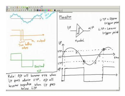
We will also understand soon why this hysteresis loop inside we will also see understand that. Now, if you give a input to it, it will generate a kind of square wave or rectangular wave. How? Say, the input is like this. So, this is input, this is output let me take a sine wave ok. So, this is input, this is time, this is 0 volt or input equal to 0. A Schmitt trigger has 2 voltage levels defined as the upper trigger point and lower trigger point.
