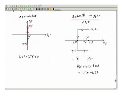
So, a small exercise for you. Can you draw the input-output characteristic of a comparator; of a comparator ok? Output versus input how will that look comparator for the comparator normal op-amp base comparator which you have shown here can you do that it is simple I will just tell you it will just look like this ok. So, and if you want to put arrows you can put the arrows like this. So, this is for a comparator.
