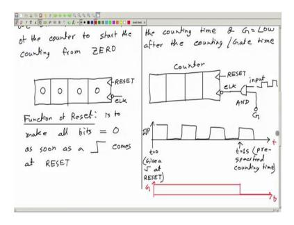
So, the input was a square wave which was applied to the clock input of a counter that is how it works.
