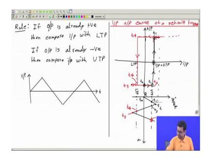
So, this is the rule actually. So, if output is already positive then compare input with can you guess? Can you guess? This is lower trigger point. If the output is already positive, then compare the input with lower trigger point ok. So, like here in this region consider this region. So, here this is positive output.
