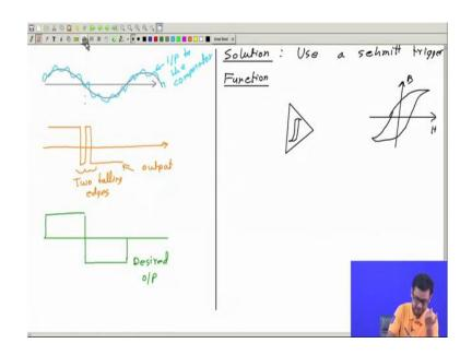
So, this blue line is the input to the comparator or op-amp and the output will be like this. In this region see; so, before this point it is positive that is fine as expected as wanted. Here it goes to negative once, then it goes to positive again, then it goes to negative once, then it stays at negative for a while up to this. So, you see that this is how the output is, but how do we want the output to be? The desired output should be like this.
