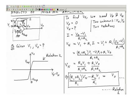
So, this is the circuit for the inverting amplifier it has one input V 1, one output V o, V P is connected to ground. I just have copied it from here we have said how to remember this circuits before fine.
