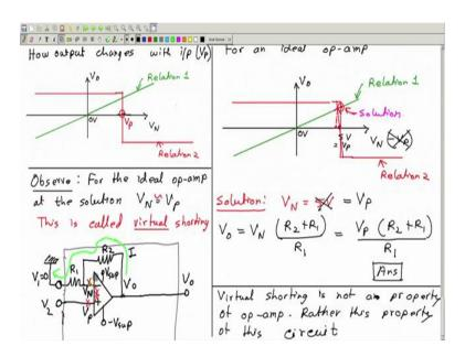
So, for an ideal op-amp, what is the modification I have to do? I have to make this line vertical as vertical as possible; and this and I can erase the previous one. So, now, the solution will be at this point. So, this is now the solution ok. So, what is the solution? So, the solution is that VN at this point VN = 5 volt but what is these 5 volts? These 5 volts is nothing but the value of V P ok.
