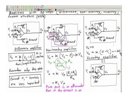
Namely, difference amplifier non-inverting amplifiers and inverting amplifier; once again we said just remember one circuit and from that you can derive the other two ok. And never ever by mistake make this plus or minus symbol wrong ok. Never swap this plus minus symbol this is very crucial I forgot to mention.
