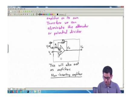
So, the rest of the circuit is an amplifier on it is own is an amplifier on it is own. So, the rest of the circuit is therefore, an amplifier. So, what we can do? We can eliminate this part ok. So, therefore, we can eliminate the this attenuator or potential divider and it will still be a amplifier because rest of the circuit will do the amplification.
