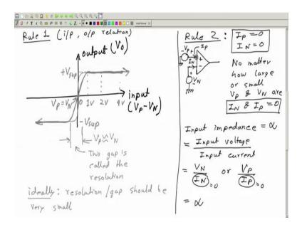
So, this is rule number 1 and then we have seen rule number 2, which is here, which says no current can go into or out of this input terminals, either of this input terminals of an op amp, which is same as saying the input impedance is infinite, because whatever voltage you apply current will be 0.
