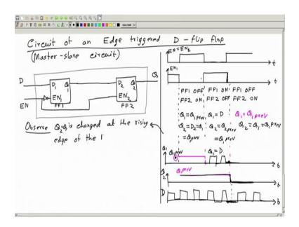
So, circuit. So, the next thing we will study is the circuit of edge triggered D flip flop and this particular circuit is called a master slave circuit. This is the name. We will understand soon why it is called so. So, what we will do is this we will take 2 D flip flops; 2 level trigger D flip flops.
