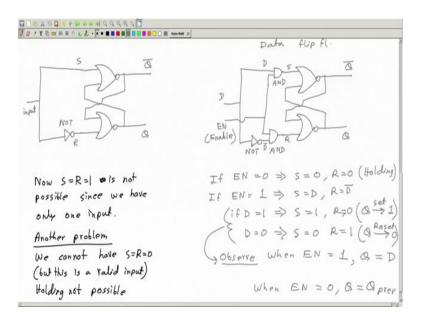
So, let me first draw the SR flip flop. Input goes to output; output goes to input ok. Now, what I will do? I will connect say NOT gate. So, this is a NOT gate or I I can also connect it, this here both will be same.
