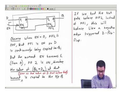
So, let me just tell the story in a different way. So, I told you the story with timing diagram ok. This is one way to verify that this is a edge sensitive edge triggered diagram, another way of understanding the story is this. So, observe that when enable is equal to 0 ok.
