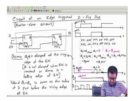
And cube is not changed. Q is that means, Q 2 is not changed when say enable is constant equal to 1 or equal to 0 or even when there is a falling edge ok. Q 2 is not changed when enable is constant or there is a falling edge negative edge at enable ok.
