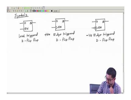
So, let us ok, before that let me tell you the symbols. So, if I draw a box with D; D means data input, Q output, enable this is also a input like this. This is this symbol is for level triggered D flip flop or data flip flop. But if I draw the same thing D Q as here, but if I put a triangle and I write enable, then this triangle symbol means this is a level triggered D flip flop.
