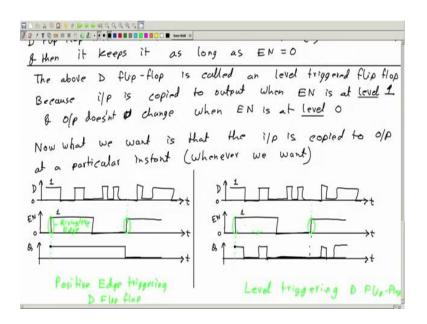
So, this D flip flop memorizes the value of the input; input D when enable is equal to 1 or enabled and then, it keeps it as long as enable is equal to 0 ok. So, if you keep the enable equal to 0; as long as you keep your enable equal to 0, if you change the value of D input output is not going to change ok. Good.
