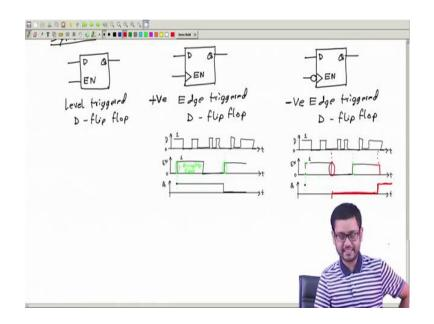
That means, this is positive edge triggered D flip flop, what we have already seen and what happens in case of a negative is triggered the only difference is that the changes occurred only during the negative edge not here ok. So, the changes occurred only during the negative edge. So, what will happen? Here Q will become 0 at this instant because data is 0.
