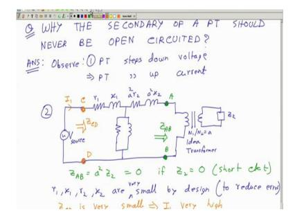
So, observe that a PT steps down voltage; so that means, PT steps up current; it has to be ok. Now, second thing second observation this is point 1 and point 2 so, this is the say this is the equivalent circuit. Then, here we have the ideal one with N1/N 2= a and if I call this impedance z 2 and here we have the voltage source V1 that we are measuring.
