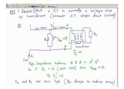
Now, so, if z 2 is equal to infinite; that means, open circuit then this is called this z AB, this is also infinite open circuit ok. So, this is infinite; so, this will imply what this current which is I 2' according to our notation. So, I2'=0. So, this side is not there at all; this part is gone, I mean from here to here this is not effectively there. And now, you observe the point 2 is that this impedance Xm and R0; Xm and R0 are very high. Why? This is by design.
