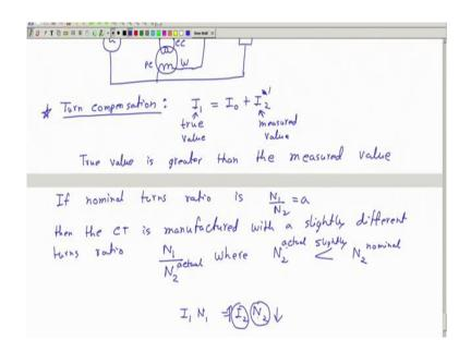
If nominal turns ratio is N 1 by N 2 equal to a, then the CT is manufactured with a slightly different turns ratio, with a slightly different turns ratio maybe like say N1/N2 new ok; where, say where I will choose N 2 new to be slightly lower than N 2 ok. If I choose this actual, so in or call this actual N 2 not new actual is slightly less than the nominal N 2 nominal ok, then what will happen this secondary current will be slightly more than the nominal value ok.
