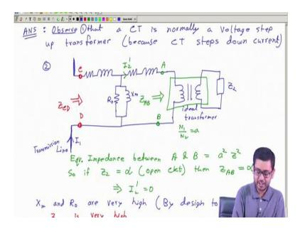
So, therefore, the total impedance say between these two points call it CD. So, let us see it from this way z CD. So, z CD is what? This impedance which is very high parallel this impedance z AB which is infinite. So, these 2 parallel combinations will be very high because this is infinite and this is also very. So, z CD; so, therefore, z CD is very high ok.
