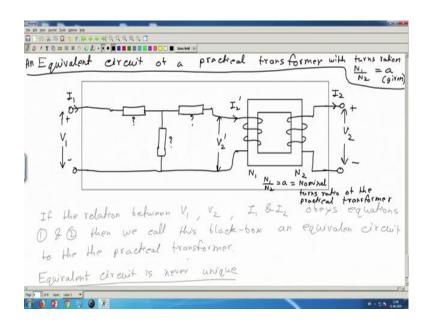
Now, next question of this is the final topic in this video is to find the equivalent circuit of a practical transformer. What do you mean by an equivalent circuit? An equivalent circuit is a circuit or is a circuit which will again have 2 ports like a transformer primary and secondary ok.
