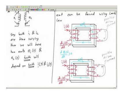
So, flux is now in the opposite direction so, this flux is in opposition to the original flux which was the cause of the induced e m f. So, this is in accordance to Lenz's law, it is not violating Lenz's law ok. So, this side will be positive, this side will be negative, you can verify that the other possibility that this is plus this is minus will violate Lenz's law ok.
