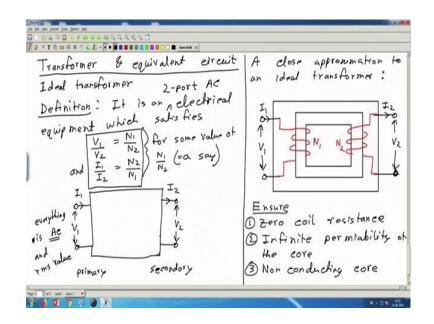
We will start this talk with ideal transformer ok, what is an ideal transformer? Let me give a definition. So, it is an I can define it this way; it is an electrical equipment electrical equipment with 2 ports. So, it is an 2 port electrical equipment like this.
