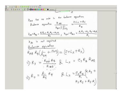
And Z C AC you can also find this way, but this is not useful because it is not going to be in the balance equation at all ok,  $Z_{AC}$  is not required so ok. Now we can put this values in this sorry in this equation. So, you can put this values of  $Z_{BC}$  from here and  $Z_{AB}$  from here in this equation to get the balance equation.
