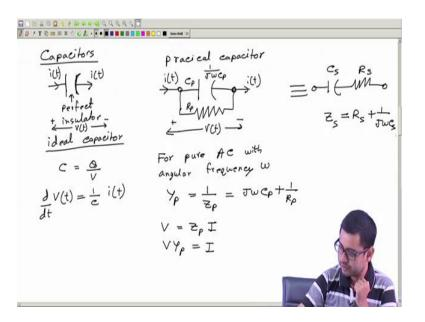
Now, an ideal capacitor which we denote with just the symbol or maybe sometimes like this ok. For this, no current can actually flow through one plate to the other through this dielectric because this is a perfect insulator ok. So, this is an ideal capacitor ok. And for this, the relationships like C = Q / V from which you get
