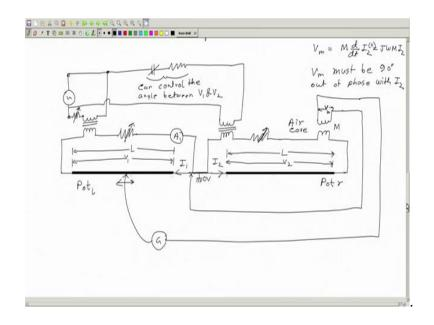
And now observe that this voltage in the secondary, call this V m. This voltage in the secondary is at 90 degree with the current which is flowing here or here I 2. V m must be 90 degree out of phase with I 2, why? Because, what is V m?
