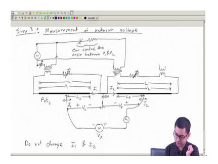
Now, final step step 3. This is the measurement of unknown voltage. So, in this phase we will still have this of course, this is always there. Here also we will have this, although we are not using it. So, you can keep it open. Here also you are not going to in this measurement phase, we are not going to use it you can keep it open, but and now we will connect the V x and we will have two jokeys.
