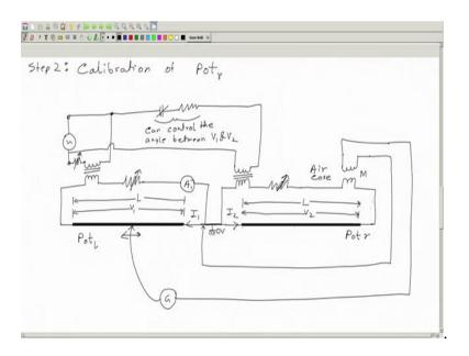
Now next step is calibration of potentiometer2. We call it Pot r. So, this is Pot r right Pot 1, Pot r. Now, for that what we will do and then we have this ammeter A1 of course, and here we will put a new equipment, what is that? That is going to be air core transformer, important that this should be air core. So, I am not drawing any core. So, this is air core transformer and so, if any current is flowing here then we will have some voltage induced
