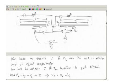
So, somehow, we have to ensure I  $_1$  and I  $_2$  are 90 degree out of phase and of equal magnitude. So, then it will actually mean that. So, this two are identical potentiometer wires.
