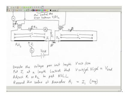
So, record the value of ammeter A1 say this is equal to I 1. So, note this value and then the calibration of potentiometer1 is done.
