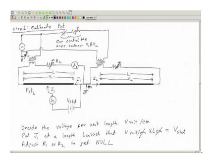
Just like we did it for the polar potentiometer, we will take a source and supply this side and this side with one side through a capacitor, resister something to change the phase angle of the respective current between the respective currents. So, what we will do is this, let me first put say a transformer here.
