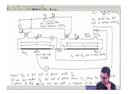
Now, this voltage V 2, V 2 is in phase with I 2. V 2 and I 2 are in same phase, why? Because this wire is resistive since the circuit is resistive. So, V 2 is nothing but I 2 multiplied by some resistance. So, V 2 and I2 are in same phase and V m and I 2 are 90 degree out of phase. Now, these two facts together, what does it imply? V m and V 2 they will be 90 degree out of phase.
