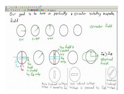
So, our goal is to have a rotating magnetic field; perfectly circular rotating magnetic. So, let us write it loosely perfectly root circular rotating magnetic field. So, what do I mean by that? So, I mean that so, if I draw the magnetic field as a vector at different time then so, this is the magnetic field at some time say t equal to 0. Then at so, they in at say t equal to 45 degree, the magnetic field should be like this.
