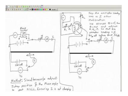
So, let me draw the AC potentiometer circuit that we had. So, this is the potentiometer wire and we have to measure a unknown voltage. So, let me have this unknown voltage VX AC. So, we connect it like this through a galvanometer, this jokey can move along the wire ok. So, we can connect it here and so, you also possibly recall that we also need a standard cell for the calibration.
