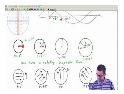
So, we may also draw the same thing like this, so at t = 0, flux lines are from left to right; at t = 45, flux lines are like this, resultant flux lines, then like this; then like this. So, the flux lines are rotating, see this is rotating. Now, so we have created a rotating magnetic field with two coils like this, which are carrying currents 90 degree out of phase, and they are placed in two perpendicular planes, they are spatially also displaced by 90 degree.
