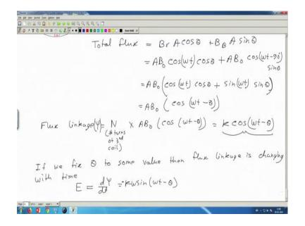
Flux linkage  $\varphi = N \times AB_0 \cos (\omega t - \theta) = K \cos (\omega t - \theta)$
