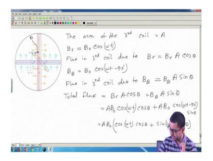
So, the 3rd coil is here ok. So, let me take this length of this coil to be much smaller like this ok. I do it on, so this is the third coil. And say the cross-section area of this coil is A. So, cross section means which area? In this diagram, this area; this area. So, that area or let me just write the area of the coil, 3rd coil is equal to A, the and it is at an angle of theta ok.
