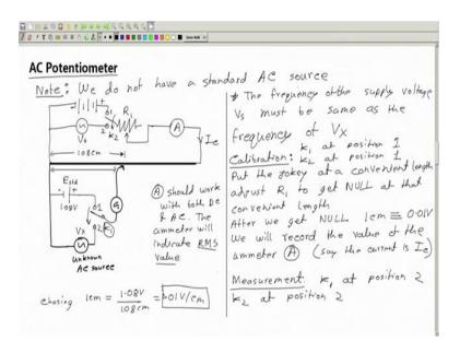
Now, the first difficulty that we have when measuring AC voltage with potentiometer is that there is no standard AC cell ok. So, we do not have a standard AC source, which we can rely on. I mean whose value does not change with any factor in I mean, so there is not as there is no such reliable AC source ok, which we can call as standard. This is the difficulty.
