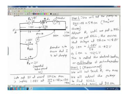
So, now the galvanometer is connected to the unknown source and this is open. So, we can have a key, with which we can switch between the standard and the unknown source. So, now, step 2. So, this is the actual measurement step. The previous was the calibration a standardization. Now, measurement, what we will do?
