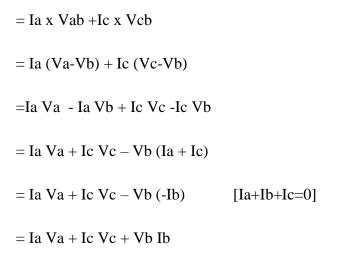
So, remember how to connect the 2 wattmeters, this is something you have to remember ok. There are some things that you have to remember, how to connect it? Connect 2 current coils in any two lines, any two lines and connect the two voltage coils between those two lines and the other unused remaining line. So, this is; so remember how to connect it? And then this derivation is straightforward ok. So, this is called 3 phase 2 wattmeter method.
