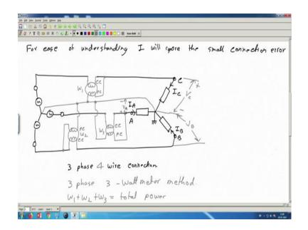
So, for now for ease of understanding, I will once again I will ignore the small connection errors which we discussed before due to nonzero current coil resistance and non-infinite
