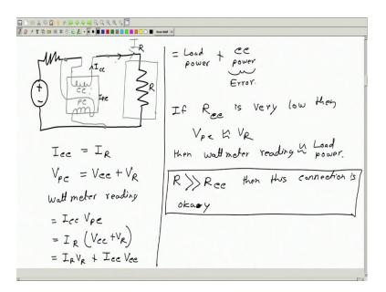
So, suppose we connect it in a different way so, that this current coil is connected after this voltage coil ok. So, we may connect this voltage coil this here ok. So, then the current coil is measuring the right current definitely Icc now is same as I R. So,
