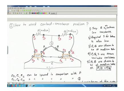
So, how to avoid contact resistance problem? We will start by drawing say Wheatstone bridge. So, this is a Wheatstone bridge with call this resistances P Q R S this is a 4 arm bridge ok.
