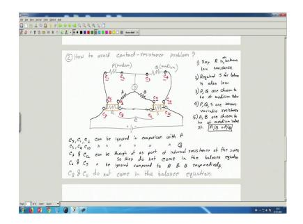
So, this C 8 and C 11 C 8 and C 11 do not come in balance equation in the balance equation and that is so, because of the principle of this bridge this circuit and this is actually true because we maintain always  $\frac{P}{Q} = \frac{A}{B}$ .
