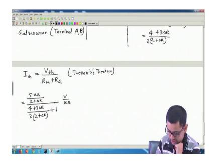
Now what will be the value of I G? I G will be nothing, but the current which will flow when we connect the galvanometer here. Now, if we connect the galvanometer here in this circuit the current that will flow through the galvanometer according to Thevenin's law
