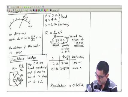
The resolution of measurement. So, what do you mean by resolution? So, possibly this is a new terminology we are introducing now. So, let us define resolution with an example. Suppose I have a meter say voltmeter which has a range of 0 to 10 volt and say it has 100 durations. So, say it has in small divisions and a total of 100 divisions or 100 markings on the scale. So, 100 divisions; that means, each division of this voltmeter is equivalent to 10 volt divided by 100 ok so, which is 0.1 volt.
