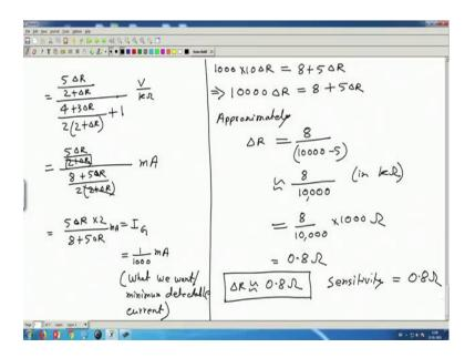
we want I G to be equal to 1 micro ampere we want this equal to 1 microampere which means ok. So, this is in milliampere 1 microampere means 1 by 1000 milliampere because. So, this is what we want or this is the minimum detectable current this is the minimum current that we can detect. So, the question we are asking that for what value of delta R this current will be same as the minimum detectable current 1 over 1000.
