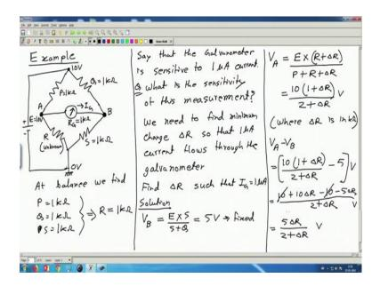
So, we will take a simple example say we have a bridge which is like this and this is the unknown this is unknown branch and say we have the detector here supply ok. So, for ease of calculation let us take a simple example where say this P is equal to 1 kilo ohm, Q is again 1 kilo ohm, R is unknown and S is once again 1 kilo ohm where we get the balance ok.
