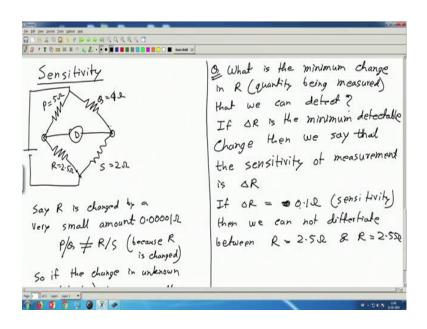
So, what do you mean by sensitivity. So, this is the bridge where we have say P Q R and S detector and the chosen value of Pi mean for this example is 5 4 and 2 5 ohm 4 ohm and 2 ohm. So, R came out to be 2.5 ohm.
