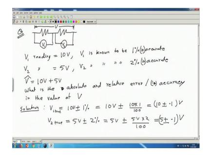
Now let us take some problems; so, question. The question is suppose I have a circuit like this, where I have 2 resistances in series and I measure the voltage across this 2 resistances with 2 Volt meters, this is call it voltmeter 1 and voltmeter 2 ok. Now
