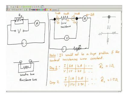
This is the low resistance we should have the potentiometer or voltmeter with infinite resistance ok; so, the here directly across it. So, this is where we will measure the voltage this can be a potentiometer or a very good voltmeter and then we will have the ammeter and here we will have the power supply. So, this is the circuit. Now, we know the you might have seen that we have resistance boxes you might have seen resistance boxes in lab.
