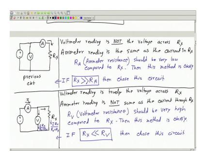
This is the previous circuit ok. Let us try another circuit. Let me put the ammeter before the voltmeter like this ok. Now it is fine. The voltmeter reading is truly the voltage across this resistance because the voltmeter is directly connected across this resistance. So, this circuit is seems like it is better ok. So, for this circuit voltmeter reading is truly the voltage across the resistance, but for this circuit it was not so.
