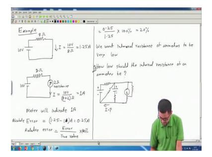
So, let us take a small example; suppose I have a circuit very simple circuit say a 10 volt source which has 8 ohm resistance in series and then some current is flowing in this branch. So, what will be this current? This current I will be equal to 10 volt divided by 8 ohm, this will be 1.25 ampere. Now, say I have an ammeter which has his internal resistance of 2 ohm for example, and I want to measure this current. So, I am inserting the ammeter 2 ohm resistance.
