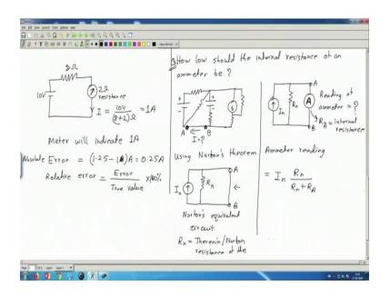
So, now how low should the internal resistance of the ammeter be to measure the current in this branch? The answer lies in the fact that according to Norton's theorem any complicated circuit can always be reduced in a simple circuit, looking from; looking from the this bit looking from the perspective of this branch between so, where we want to measure the current.
